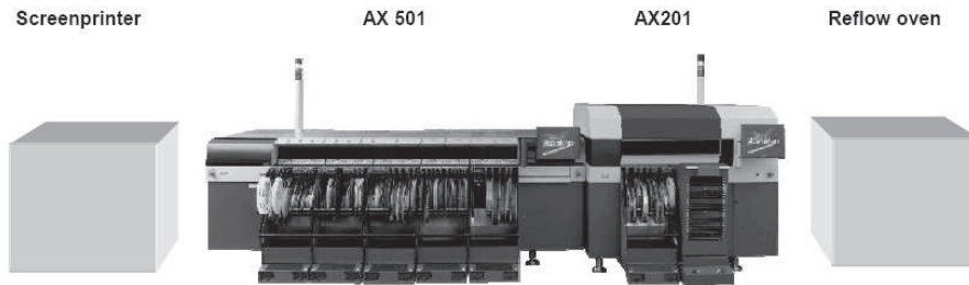
Figure 8.1: SMT process steps.
